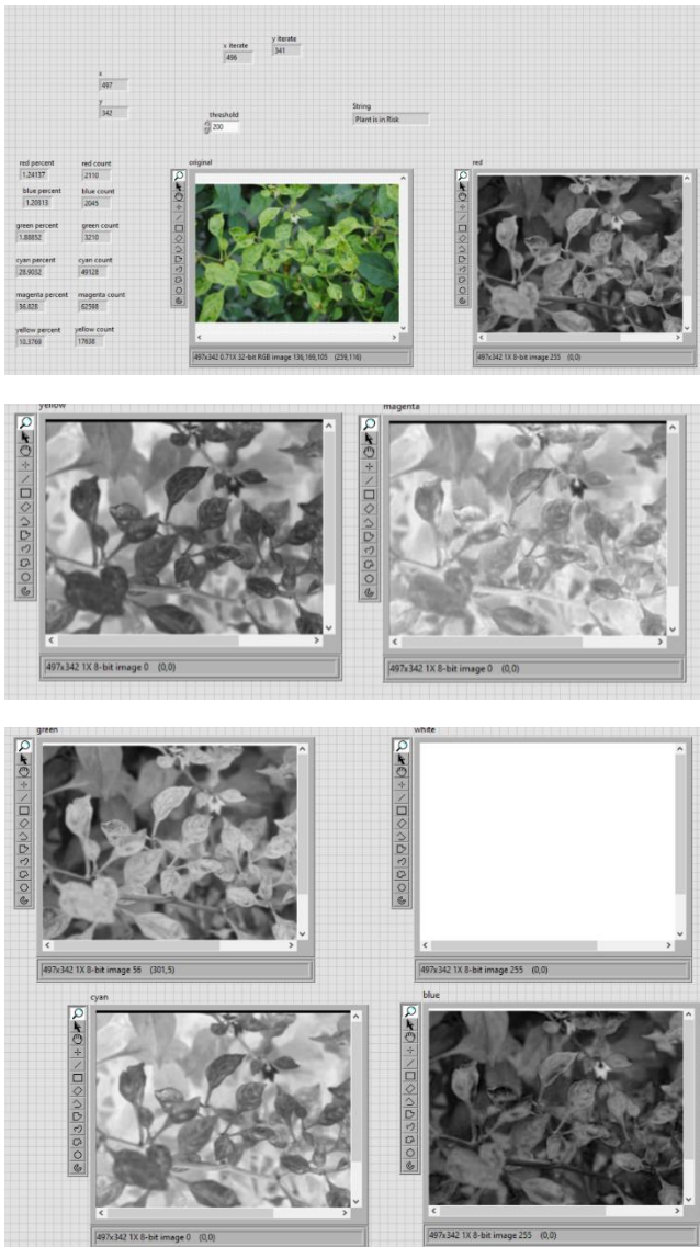
Figure 4.2: Color plane extraction and the percentage of RGB and CMY present in the leaves
