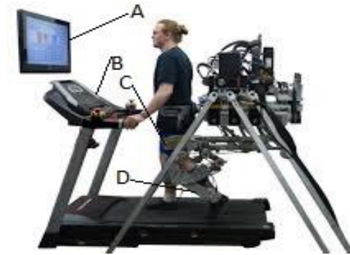
Fig. 5. ALEX(University of DELAWARE) : A. Visual feedback device, B. Treadmill, C. Leg thigh, D. Leg shank.
