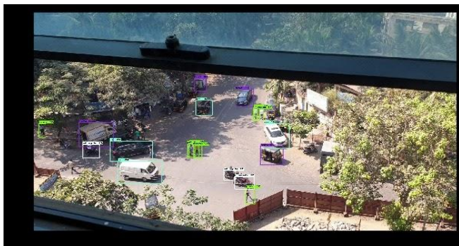
Fig. 4. Sample frame from our traffic recording showing identified vehicles and their types
