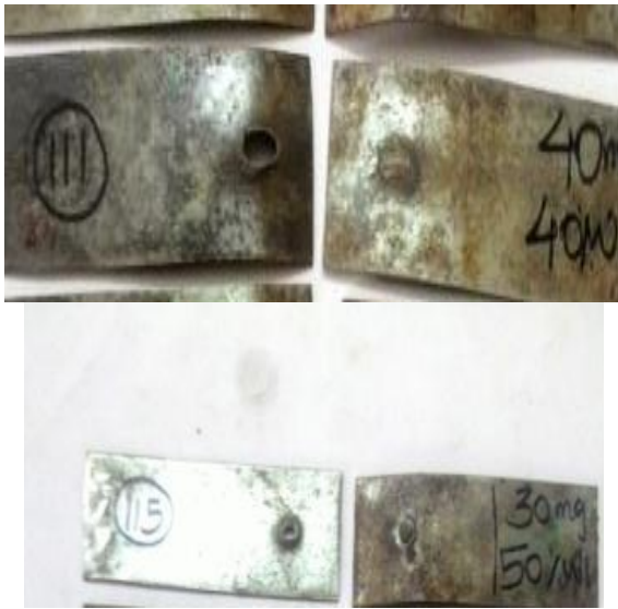
Fig 6 – Failure modes in spot specimens: Button pull out and interfacial
