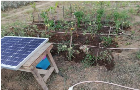
Figure 6. The setup of the Plant Monitoring System for Vegetable Growers. The solenoid valve is connected to a water source then distributes it to the drip line hose that waters the plant sideways.
