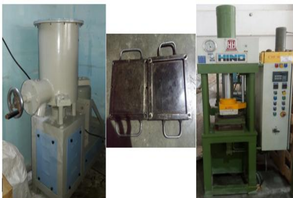
Fig. 1. Experimental Equipment (Agglomerate, Mold, and Compression Molding Machine respectively) utilized in the process of preparing the composite sheets
