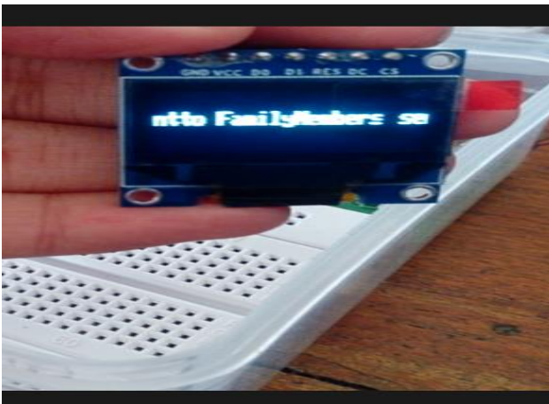
Fig. 5.OLED displaying the action performed by push buttons.
