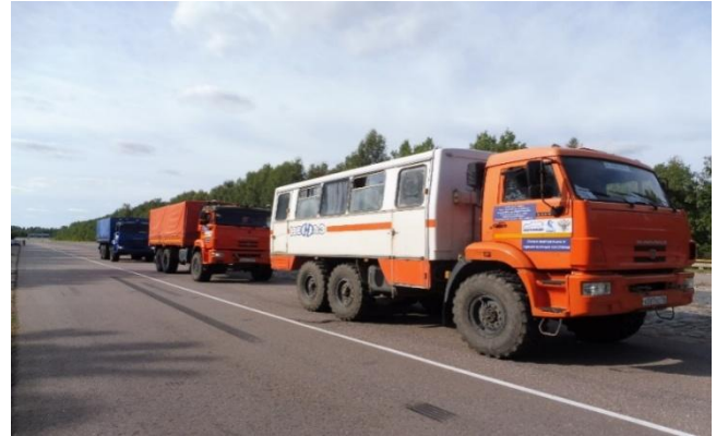
Fig. 1: General view of unmanned vehicle convoy with master manned vehicle
