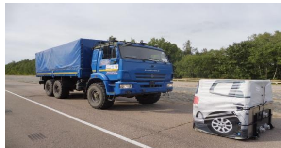
Fig. 6: Unmanned KamAZ braking in front of EuroNCAP Vehicle Target
