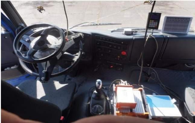
Fig. 3: Instruments in unmanned KamAZ cab
