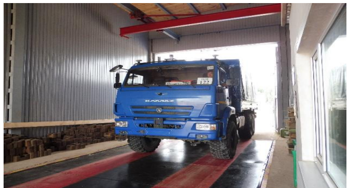
Fig. 2: KamAZ-43118 on truck scale of test track
