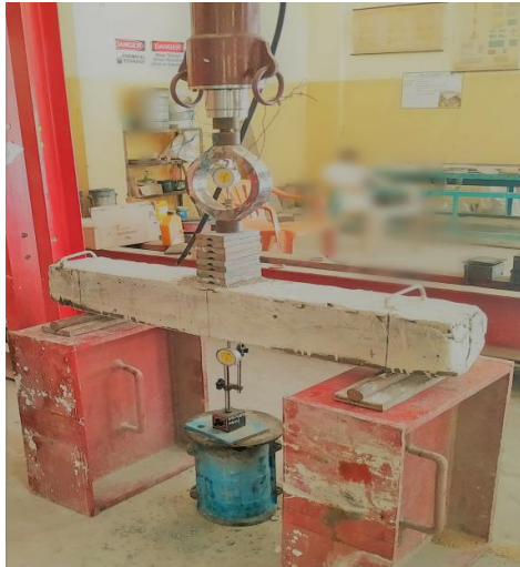
Fig.8. Experimental set up and placing of beam
