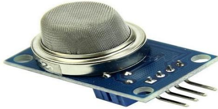
Figure3: Structure of MQ2 gas sensor
