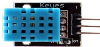
Figure2: Structure of DHT1
