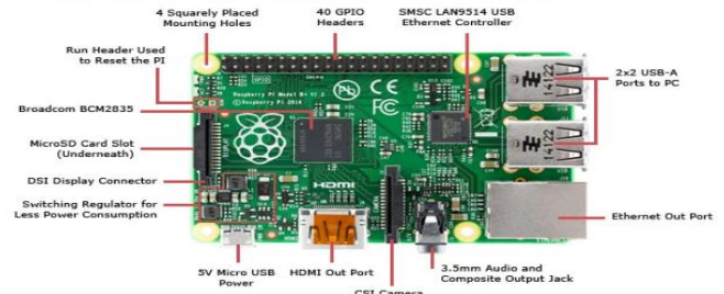
Figure1: Structure of Raspberry Pi 3 b+
