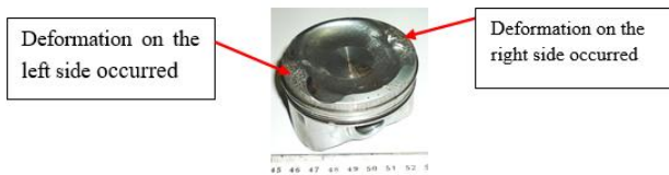
Fig. 2. Deformed Piston on 1000cc engine capacity sedan
