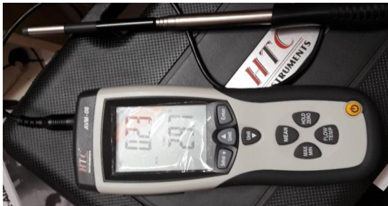
Figure 5. HTC AVM -08 Hot Wire Anemometer
