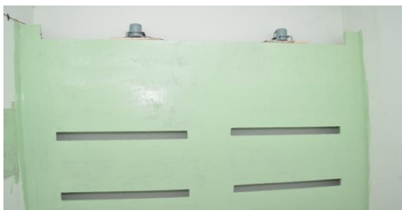
(c) Third Arrangement with fans in active mode double slot (M&D) uncovered
