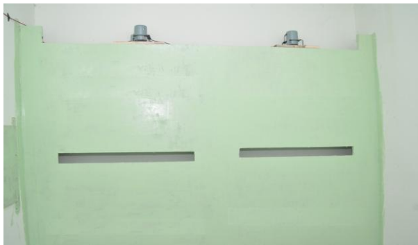
(b) Second Arrangement with fans in active mode & center slots uncovered
