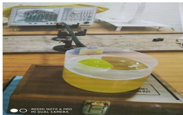
Fig .10 Experimental set-up Breast Phantom UWB Antenna with and without tumor connected to Vector Network Analyzer (VNA)
