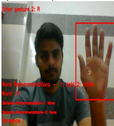
Figure 3: model recognises gesture1 as alphabet 'r' and recommends words such as 'right' and 'rather'. User can choose any of the recommendations as per his need with ease of 1 time-step. If user wants to spell different words such as 'route'. Then user can show second gesture to system.
