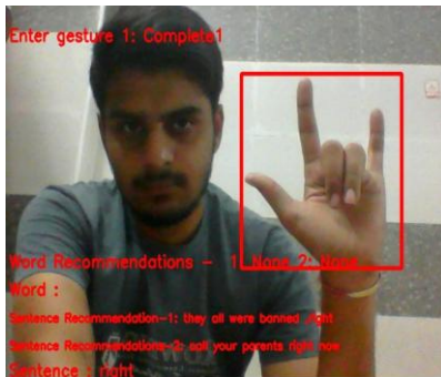
Figure 4: If user just spelled word 'right' using pyttx3 (text to speech converter). The system recommends sentences (such as 'call your parents right now') that user would like to spell before entering first gesture of second word. But we used bigram (last 2 words for sentence recommendations).
