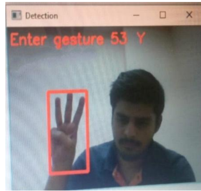
Figure 2: weight pruned Faster-RCNN detecting the hand and classifying it as Alphabet 'y'
