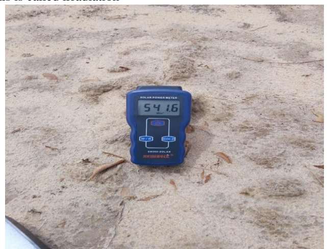
Fig.4. Solar Radiation experimentally using radiation pyranometer
