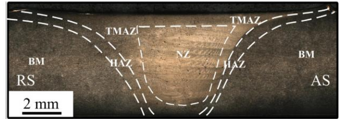
Figure 8: Macrograph of 5A06 aluminium alloy joint by FSW with highlighted the different zone [28]
