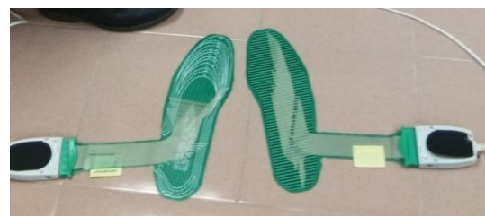
Fig. 1. A set of sensor pad use to detect pressure when foot is contact onto it
