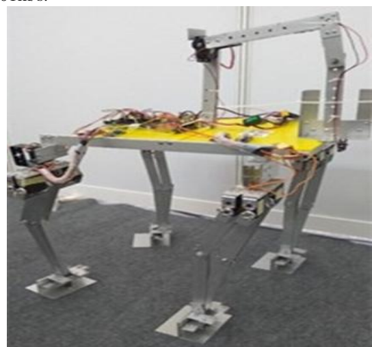
Fig. 11 Quadrupedal robot with second leg design and extension mechanism system
