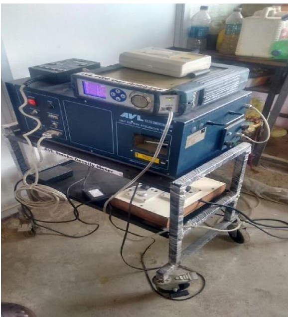
Figure 2: Five gas analyzer
