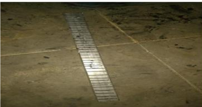
Figure 10. Slots made in stainless steel pipe
