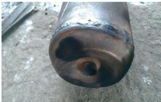
Figure 3. Rear end welded after stocking
