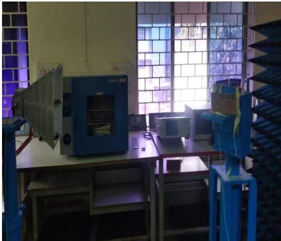
Fig. 4(a) Setup for the measurement of radiation pattern and gain
