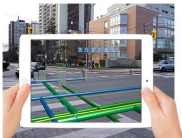
Fig.5. Combined GIS data with augmented reality to display a water distribution network 1 .
