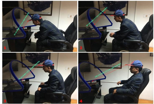
Fig.4. The experiment conducted under 111 lux light intensity with different distances 25cm, 50cm, 75cm and 100cm represented by numeric 1-4 respectively.
