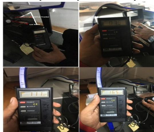
Fig.6 Lux meter readings under different light intensity.
