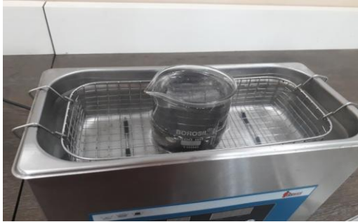
Figure 3: Ultrasonic agitation of mixture of PoE oil and CuO nanoparticles
