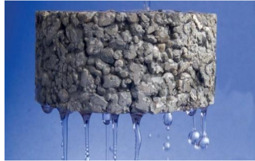
Fig. 2 Pervious concrete water infiltration
