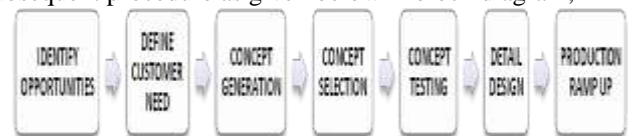
Fig2.1: Thought development procedure block diagram
