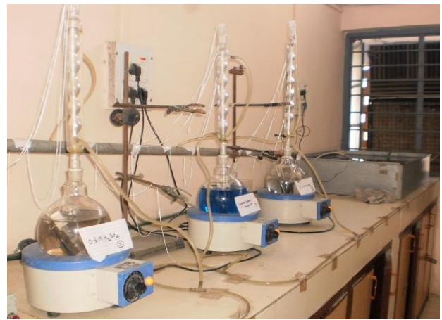
Fig. 12 Experimental set-up for 3 different chemical exposures of tensile samples
