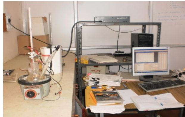
Fig. 17 Experimental set-up for corrosion test of parent metal 409M FSS
