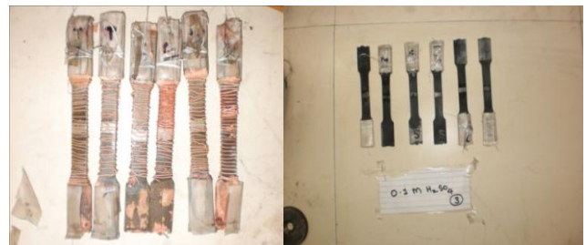
Fig. 12 Experimental set-up for 3 different chemical exposures of tensile samples
