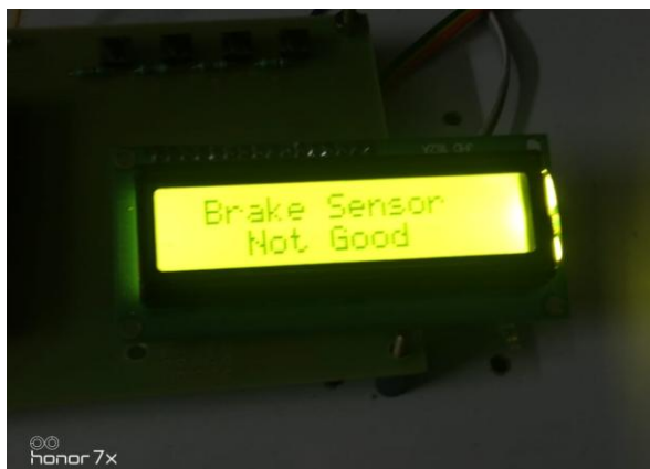
Fig. 9. Output of Brake sensor- abnormal condition
