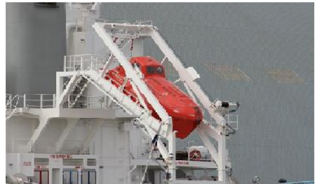
Fig.1 Figure showing free-fall lifeboat placed on its launching rail
