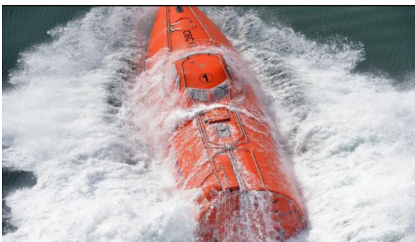
Fig.2 Figure showing the slamming effect of free-fall lifeboat.
