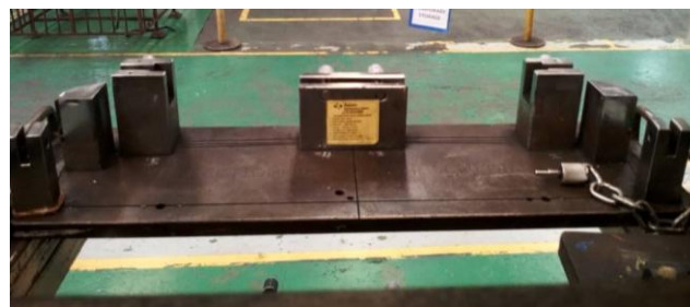
Figure 3: Gig used to determine the final dimension of spring steel stabilizer bar
