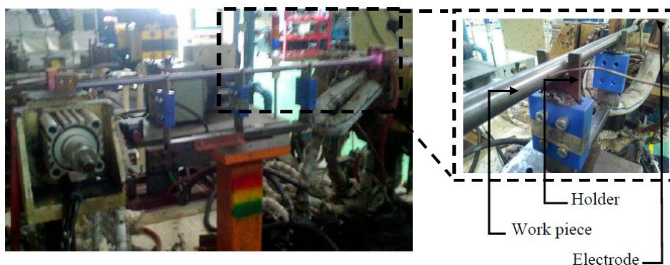
Figure 1: Experimental setup; resistive heater machine
