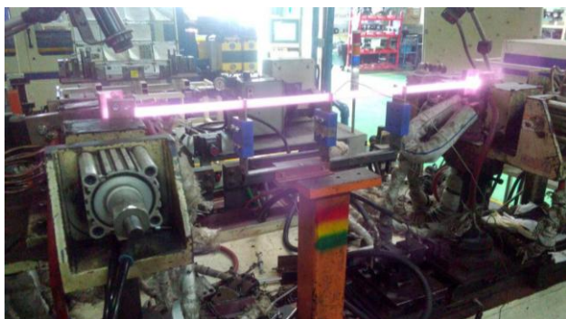
Figure 2: Resistance heating process of spring steel
