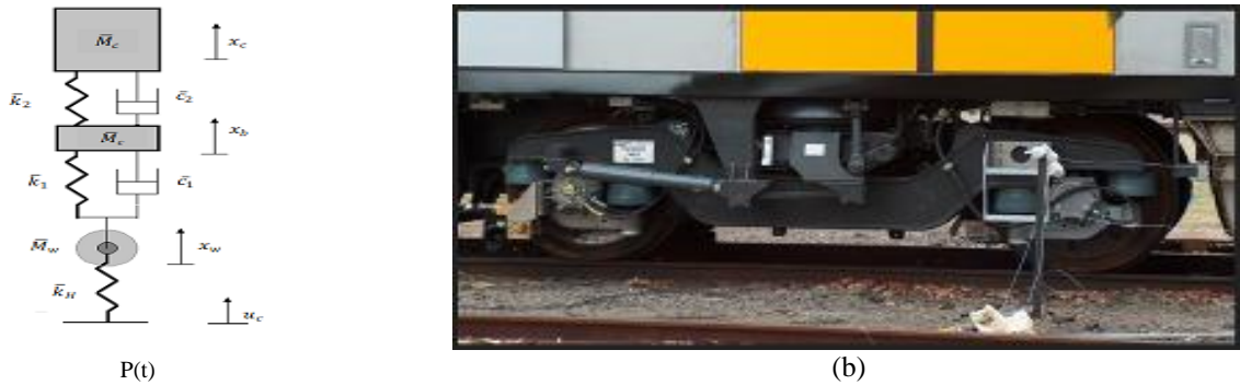
Fig. 1(a) Quarter Car Model (b) Rail Bogie System [5]
