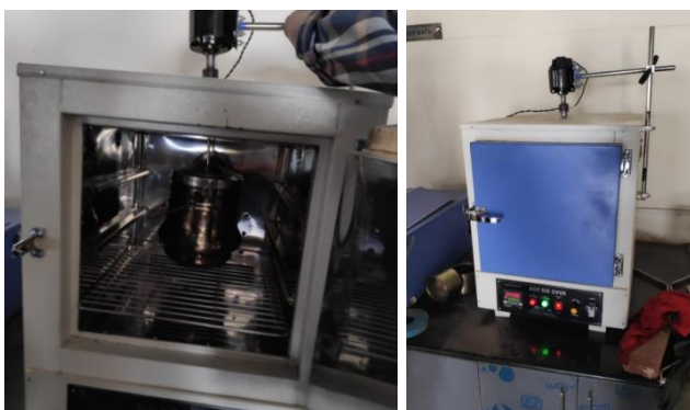
Figure 1: Mixing crumb rubber and bitumen with mechanical stirrer with oven
