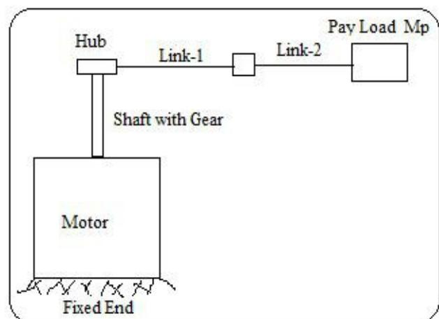
**Figure 1. Schematic Diagram of 2 Flexible Links**
