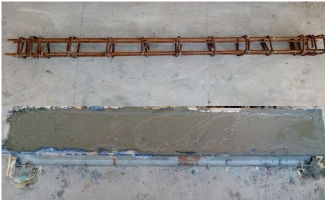
Fig.4: Mould of specified dimensions and reinforcement details.
