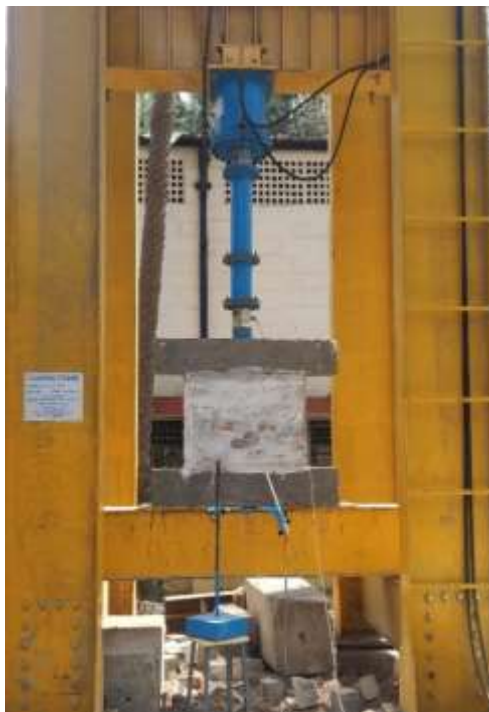
Figure 8: Original load Setup of Brick Wall
