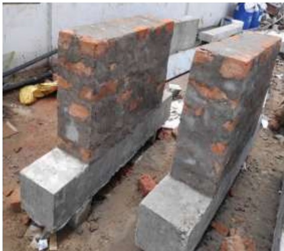
d) Unreinforced and reinforced brick wall
