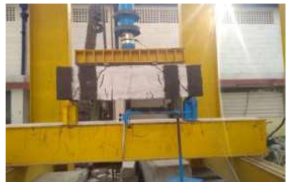
Fig. 15: 2-Stripped CFRP wrapped beam
