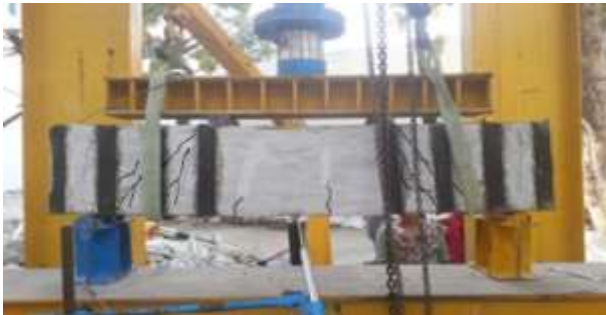
Fig. 11: 4-Stripped CFRP wrapped beam
