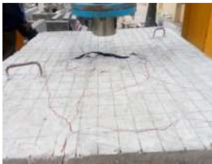
Fig. 10: Cracks on the slab after loading
