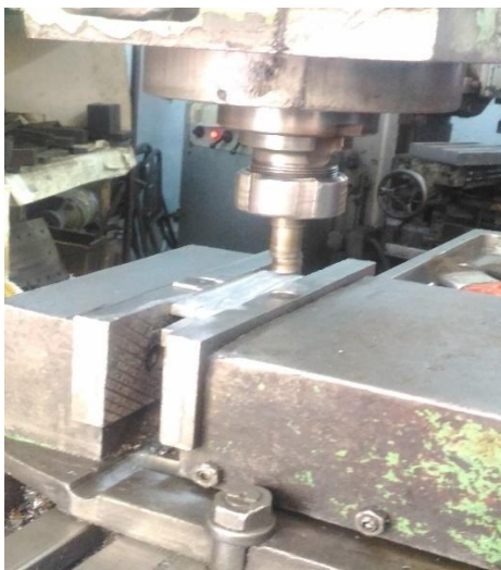
Fig 1: FSP Machine with tool set up
