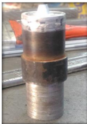
Fig 2:PCBN tool with conical pin
