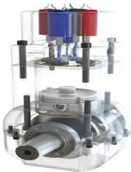
Fig: 3.1 The Primary Piston is Mounted on the Secondary Piston
