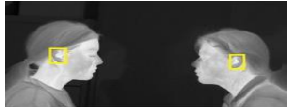
Fig.5. Sample thermal (MWIR) profile images of multiple subjects where the ears are left and right 'detection results' [29].
