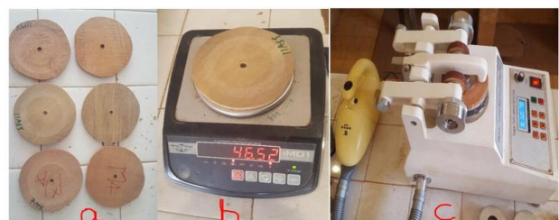
[Fig.3: (a) Abrasion Test Specimens, (b) Balance and (c) Abrasimeter]
