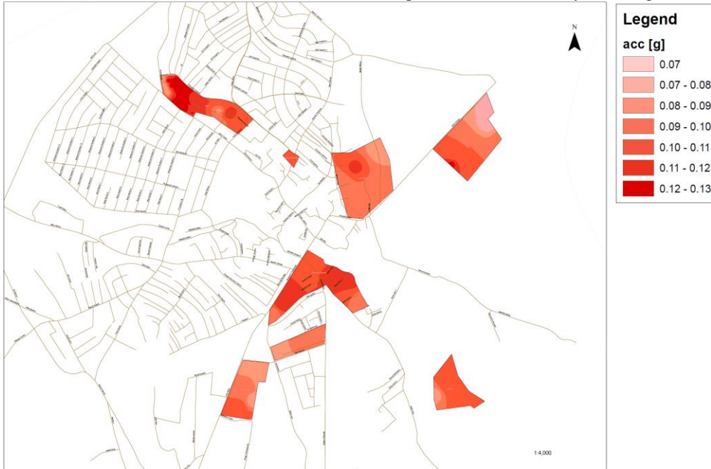
Fig. 8 Spatial Distribution of Maximum Acceleration at Foundation Depth (-2.0 m) TDLR 95 Years
