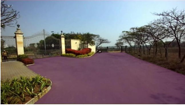
Figure 6 Output of YolactEdge Model (Road Instance Segmented)
