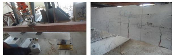
Figure 3.2 Loading of control beams
